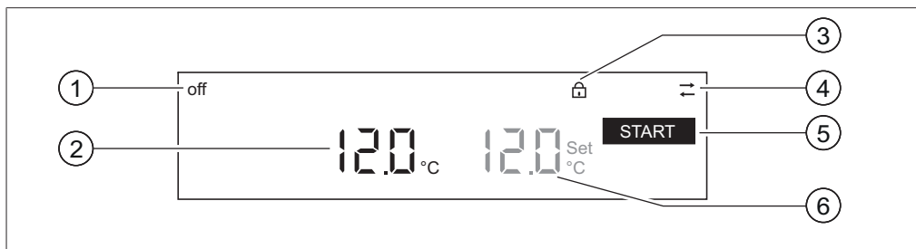
Fig. 4: Temperature display on the control panel
