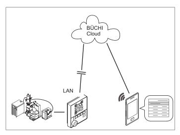
BUCHI Connect Scenario using distillation system, using smartphone, cloud and server.
